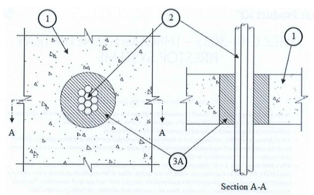
1. **Floor or Wall Assembly** — Min 150 mm (6 in.) thick reinforced lightweight or normal weight (1600-2400 kg/m³ or 100-150 pcf) concrete floor or wall. Wall may also be constructed of any UL Classified **Concrete Blocks\***. Max diam of opening 150 mm (6 in.).
